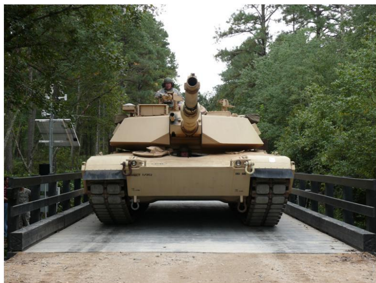
Figure 2. M-1 Abrams tank (71 tons) crossing the RTCL bridge T85-18 at Fort Bragg on September 18, 2009.
